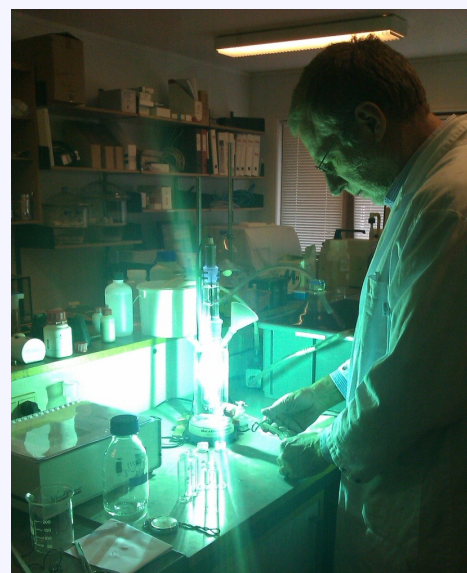
Figure 4 – AOP tests for removal of trace organics from RO permeate
