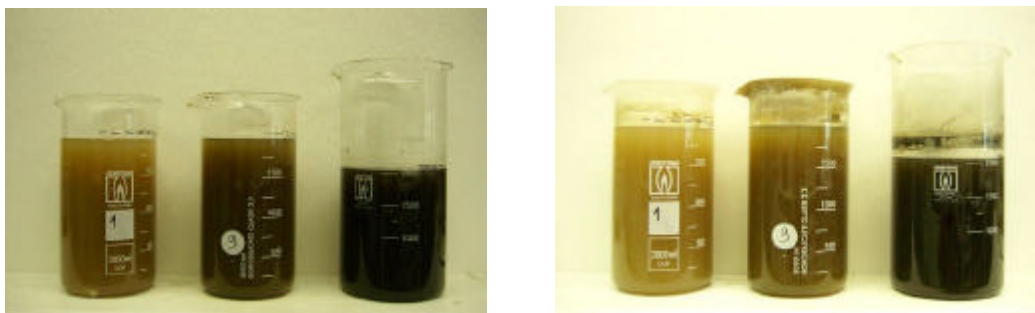
Figure 3: Batches at the beginning (left) and at the end (right) of the Zahn-Wellens test
