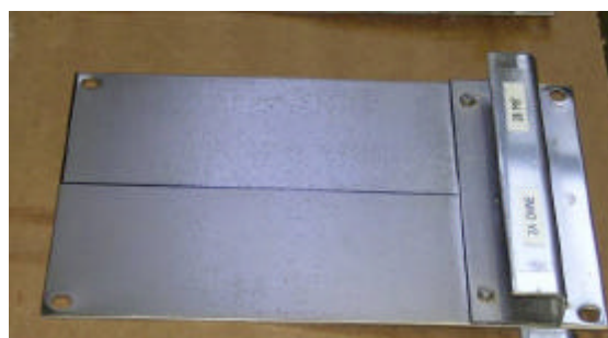
Figure 4: Steel panels (left – uncoated panel, right – panel with normal and Ag-doped colour)
