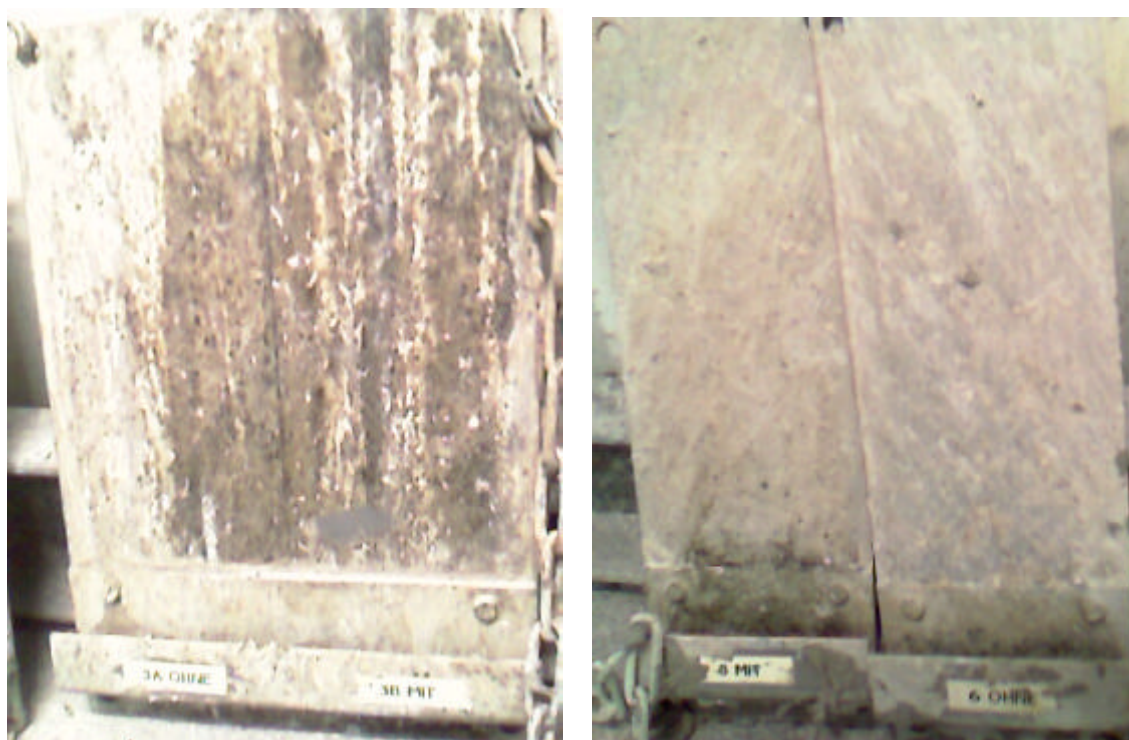
Figure. 12: Growth of biofilm and a mixture of fibre and slime on the panels
