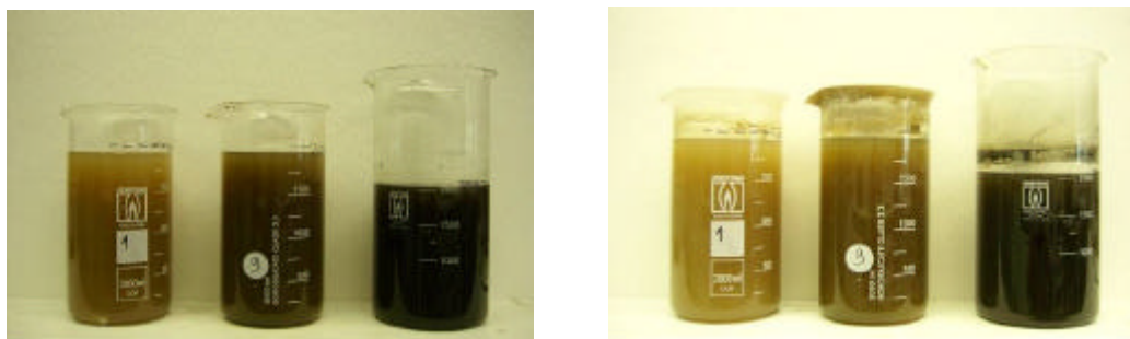
Figure 10: Batches at the beginning (left) and at the end (right) of the Zahn-Wellens test
