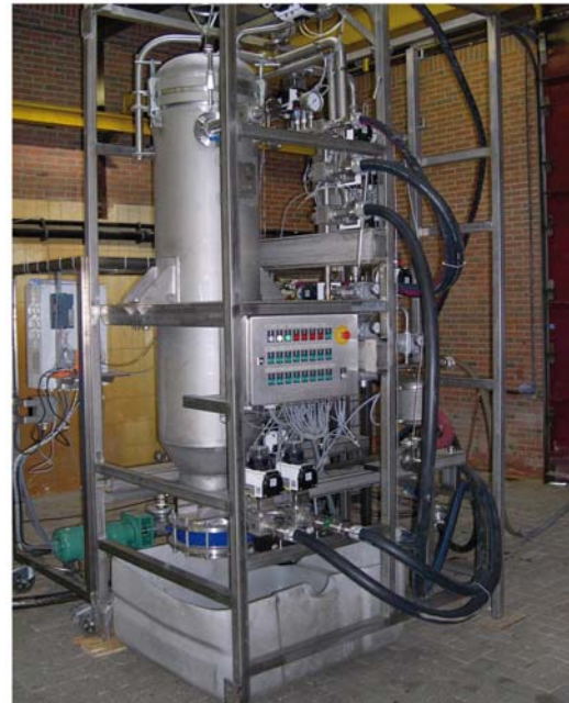
Figure 3: Pilot in paper industry. Second frame with PTS-WDCD filtration unit
