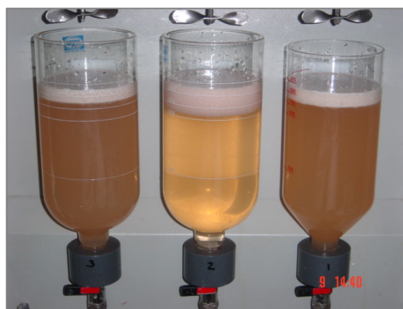
Figure 3.- Characterization of the efficiency of different chemical treatments in a lab scale DAF unit.
